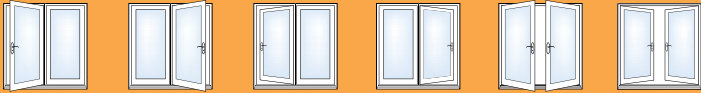
Center Hinge, Swing Left, Out Center Hinge, Swing Right, Out Center Hinge, Swing Left, In Center Hinge, Swing Right, In French Hinge, Right or Left Active Handle, Out French Hinge, Right or Left Active Handle, In
